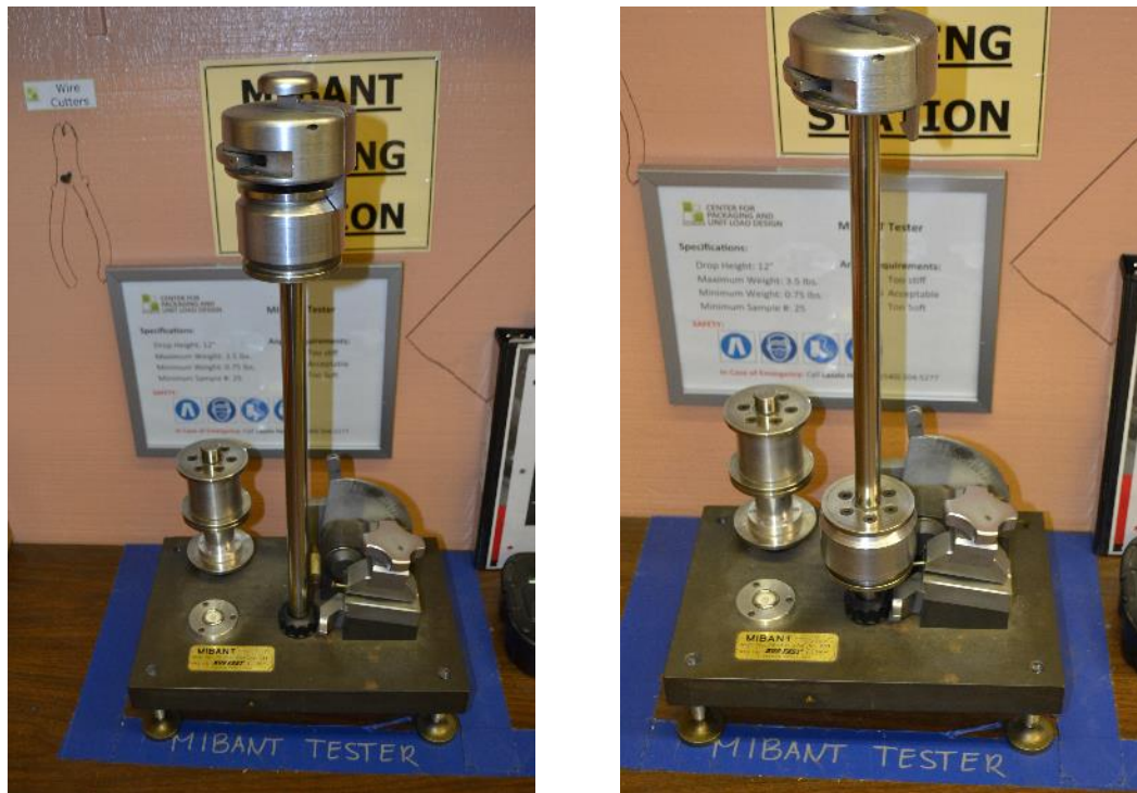
Figure 2 Experimental setup for the MIBANT test.
