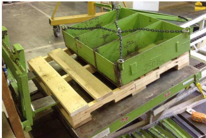
Figure 4 Experimental setup for incline impact test on pallet edges.
