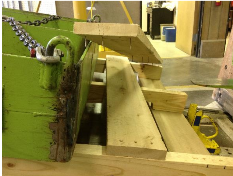
Figure 5 Representative mode of failure of the investigated pallet design during the incline impact test on pallet edges.
