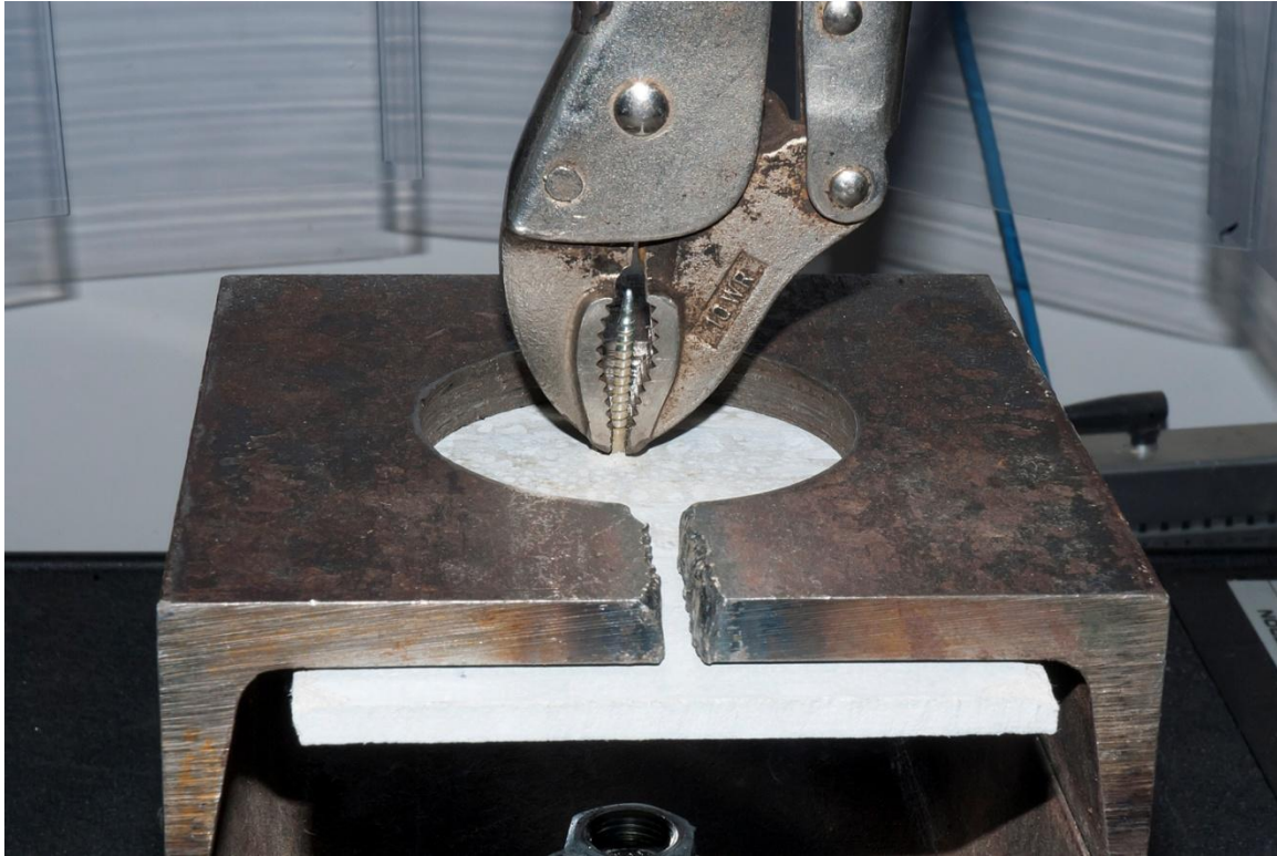
Figure 2. Typical Screw Pull Through Setup
