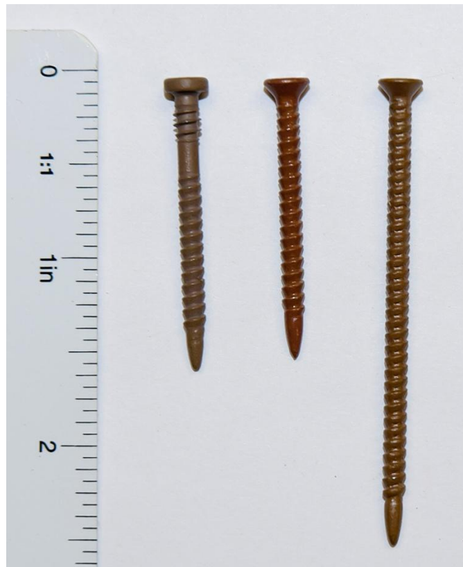
Figure 1. Typical fasteners used for pull-through testing (1.5 inch PPG Flathead, 1.5 inch PPG Combo TH and 2.5 inch PPG Flathead, left to right)
